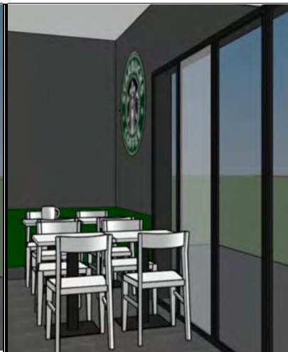
Figure 8: One of the Glazing Panels in Opaque State.
