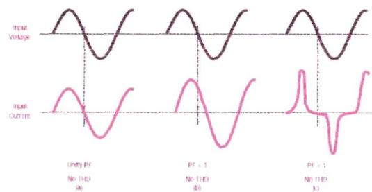
Figure 2: Relationship of AC input voltage and current
