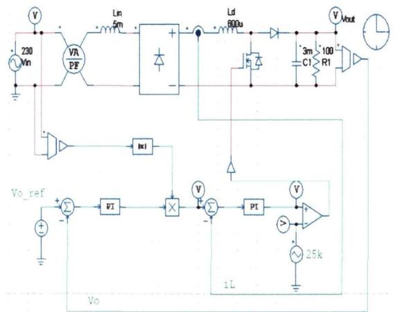
Figure 7: Simulation for active PFC (boost converter)
