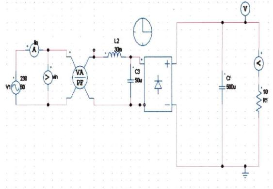
Figure 6: Simulation for Passive PFC
