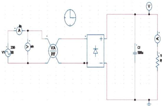
Figure 5: Simulation for non linear load without PFC
