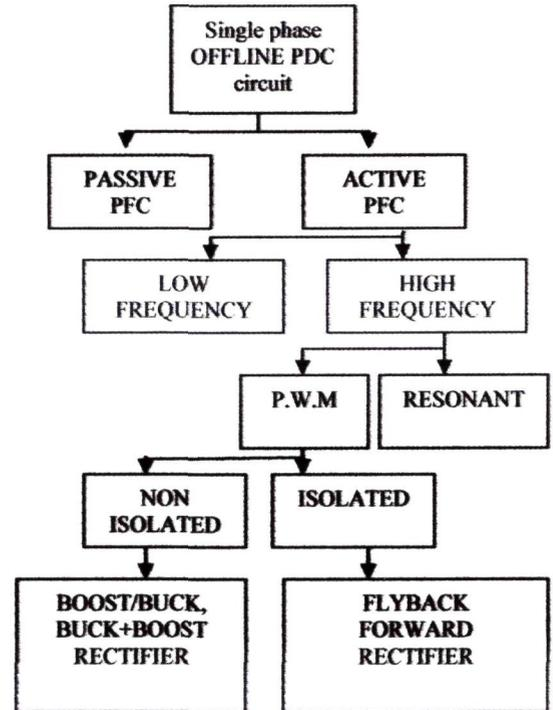
Figure 4: Single phase offline PFC topologies
