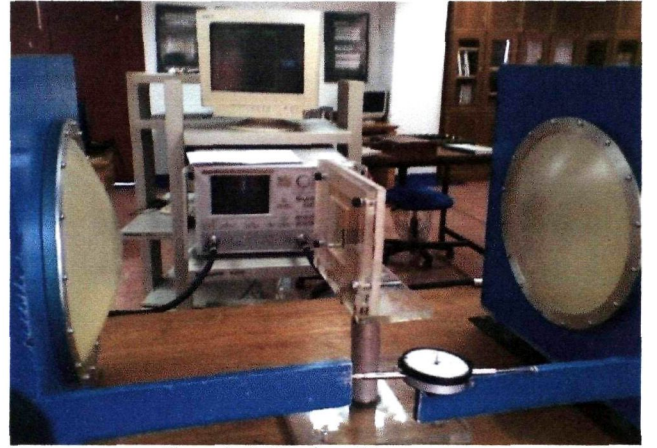
Figure 3: Calibration of S_{11} parameter
