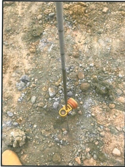
Figure 3.5: Reflecting the exact point with prism
