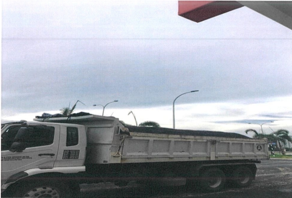
Figure 2.7 – Shows the lorry carries the Asphaltic Concrete Wearing Course ACWC14
