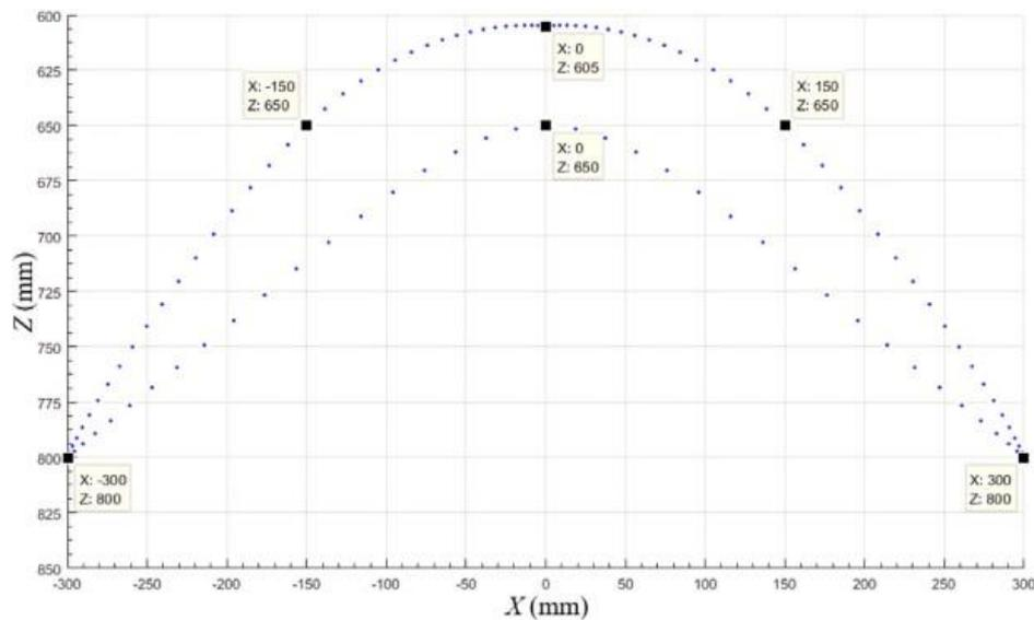
Figure 3. Trajectory Planning by Cubic Polynomials
