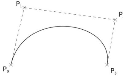
Figure 2. Bezier Curves with four control points
