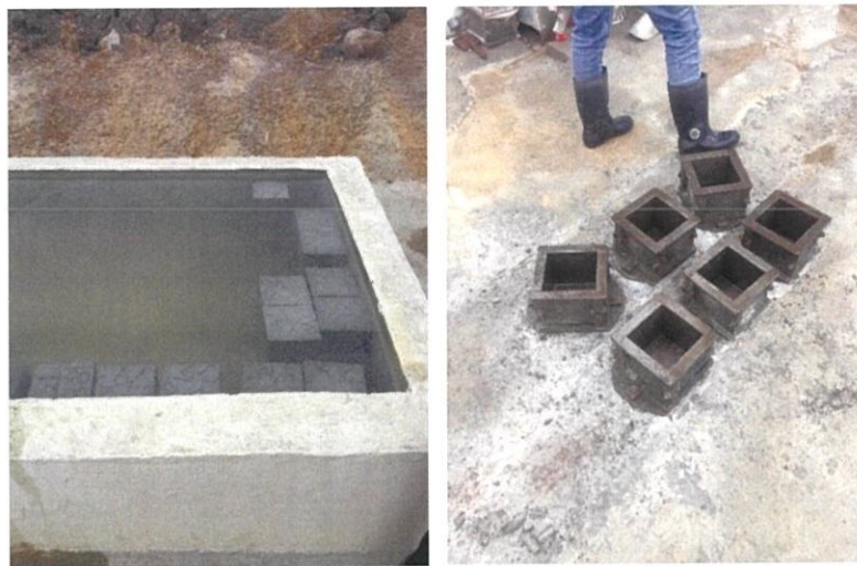
Figure 3.13 Conducting the cube test
