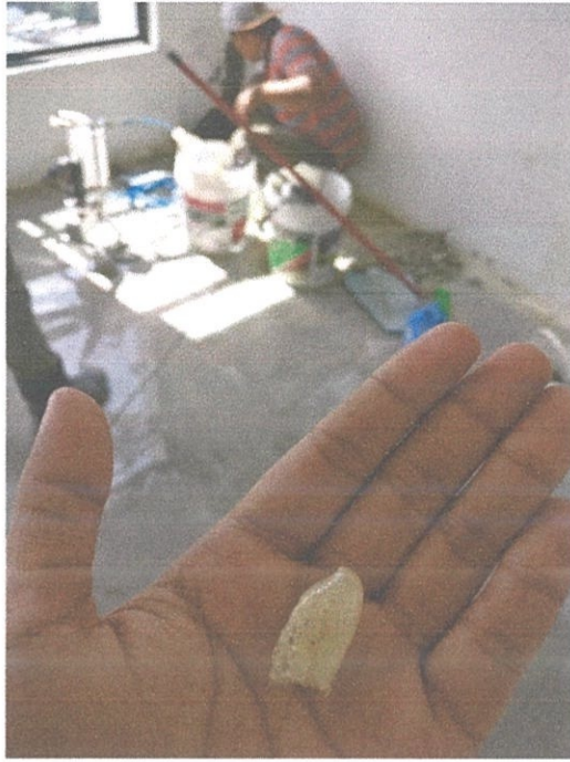
Figure 3.41: The PU once it has hardened up
