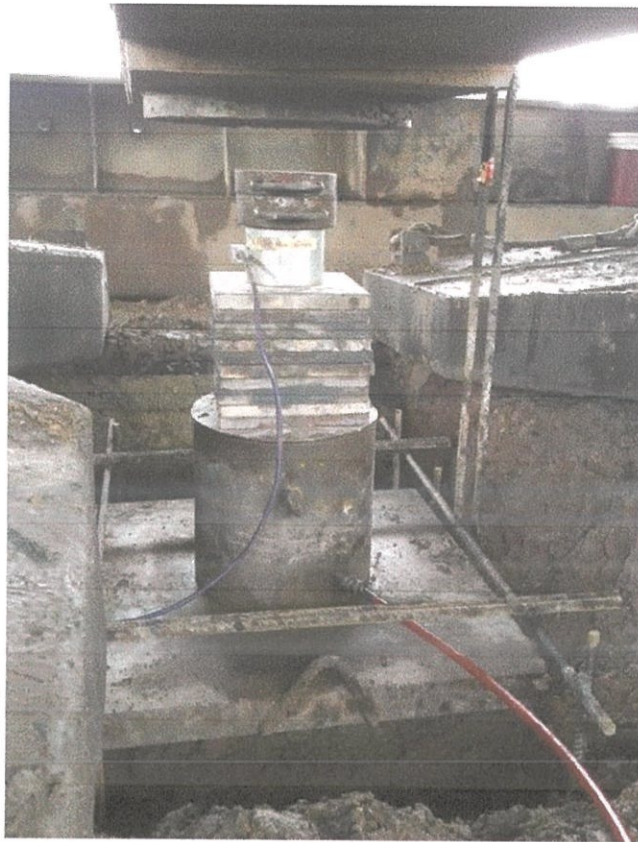
Figure 3.30 Hydraulic jack and loaded jack fitted with pressure gauge.
