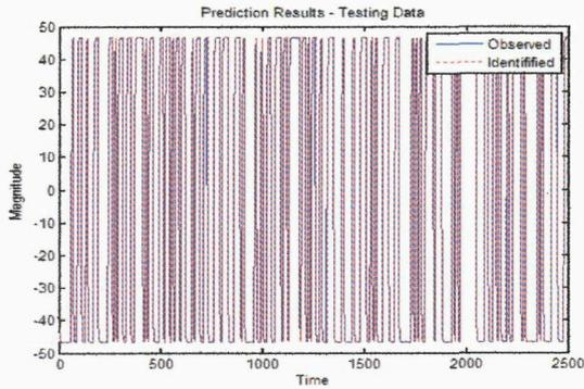
Fig.9 Identification result for testing set. Solid line indicates actual (observed) output; dotted line indicates NARX model (predicted) output.
