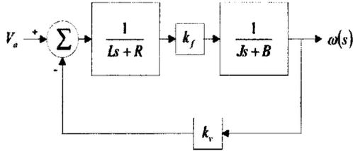
Fig.4. Block representation of DC motor model.
