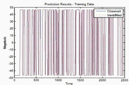
Fig. 8 Identification result for training set. Solid line indicates actual (observed) output; dotted line indicates NARX model (predicted) output.
