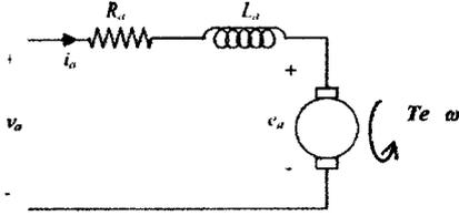
Fig 1. A schematic diagram of the permanent magnet DC motor
