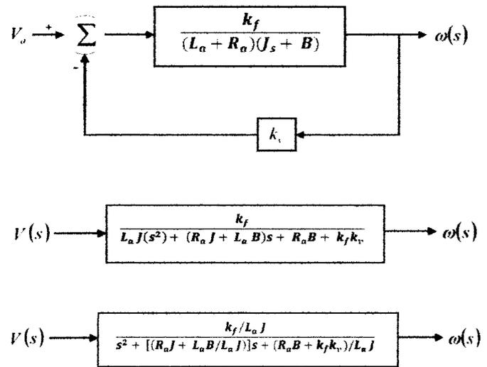
Figure 2. Overall transfer function for the DC Motor
