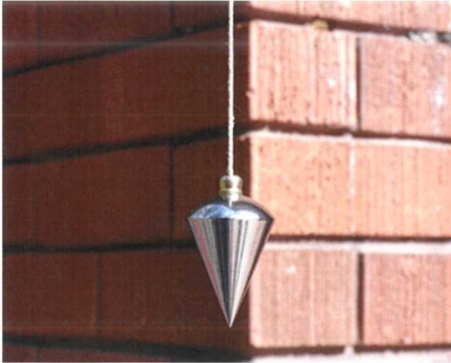
Figure 3.4 String that are attached with plumb-bob used in a setting out process Source: KITACON SDN BHD brickwork slide show (2019)
