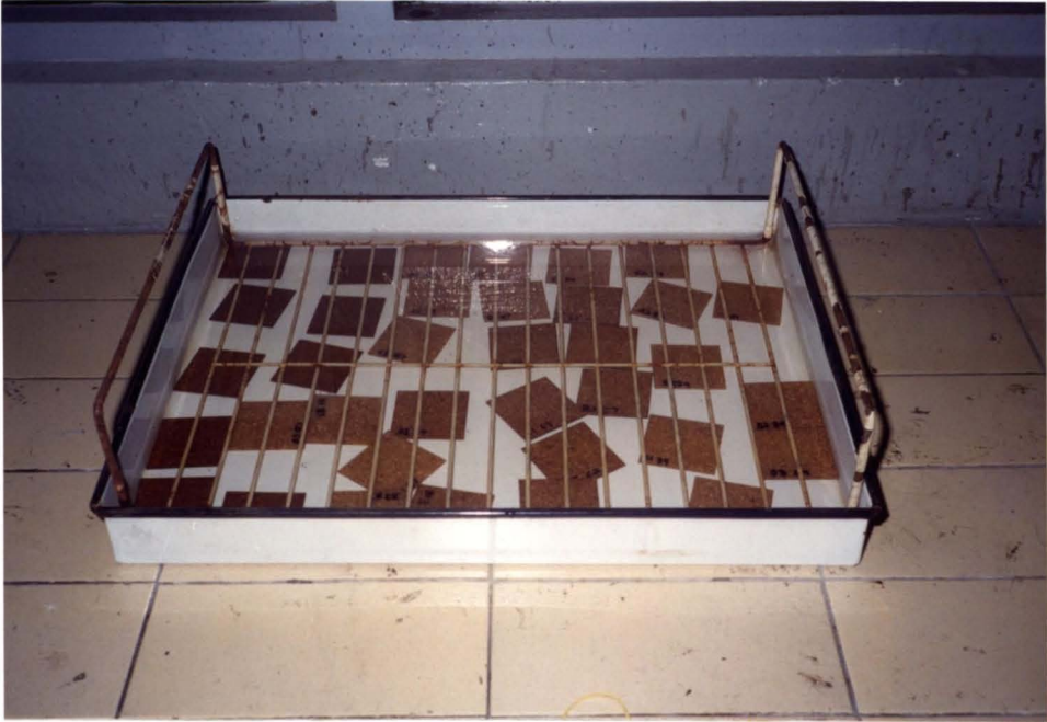
Plate 8: Water Absorption Testing
