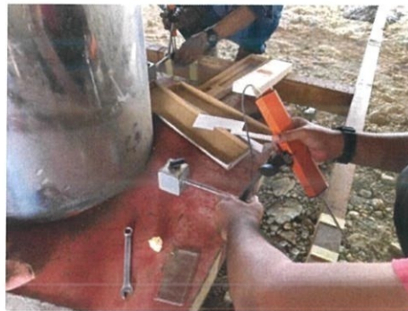
Figure 3.20: Calibrated dial gauge is placed at every corner of reference beam
