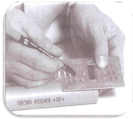
Figure 4.9 Marking process (source: Tetuan Yeo Plumber Sdn Bhd)
