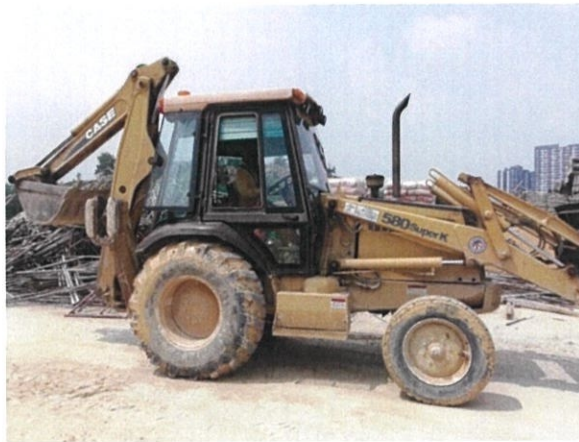
Figure 3.21: Backhoe with a digging bucket.
