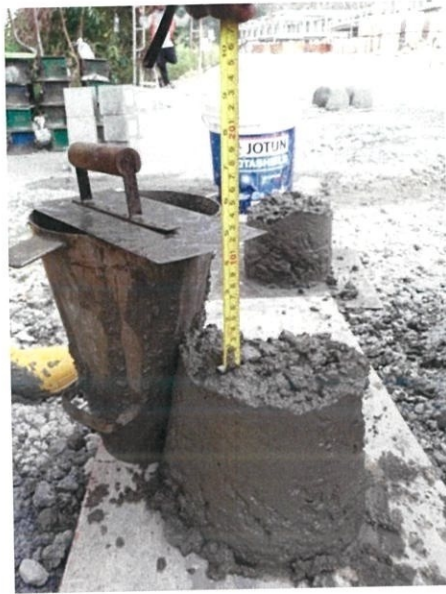
Figure 3.15: Reading of slump test was measured.
