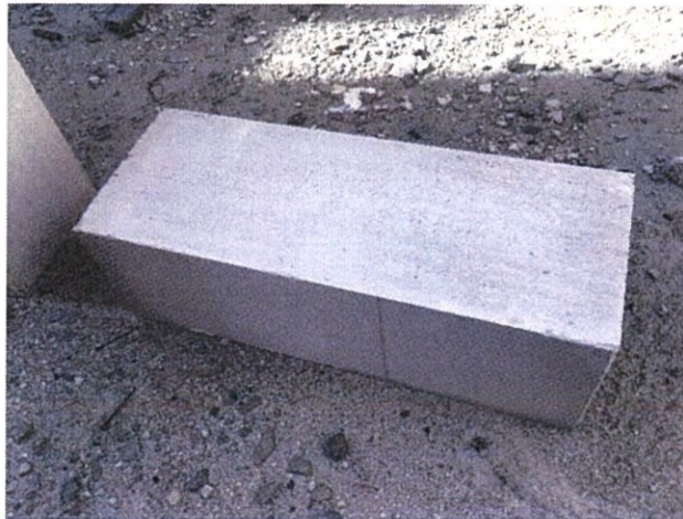
Figure 3.12 AAC block with size 225 x 600 x 200
