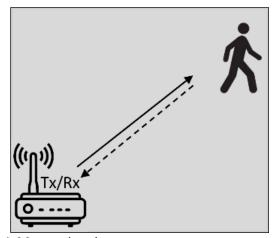
Fig. 1. Monostatic radar.
