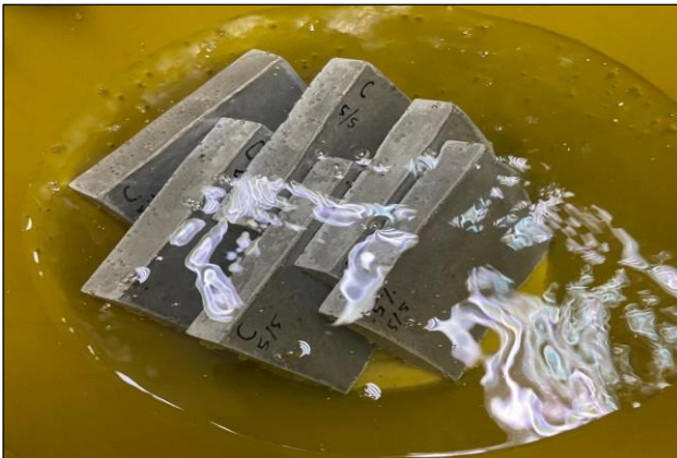
Figure 1: Cement-eggshell composites were immersed in water for 14 days
