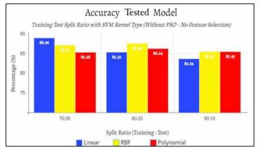
Fig. 3. Comparison of algorithms performance without PSO - Feature Selection
