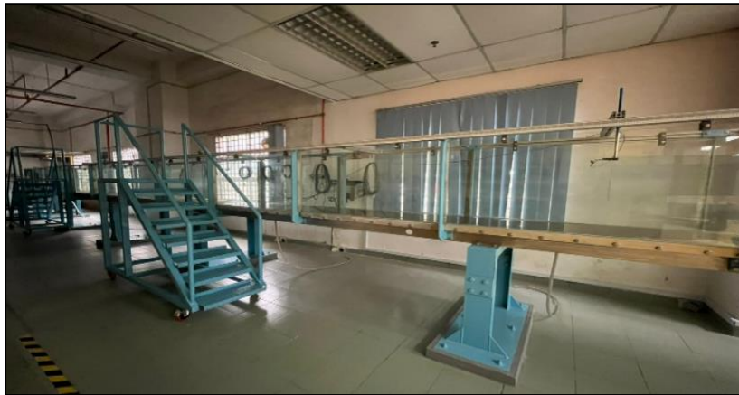
Figure 3. 2D Wave Flume used in the laboratory assessment
