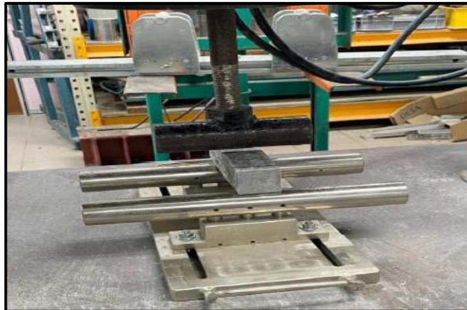
Figure 5. Flexural strength testing
