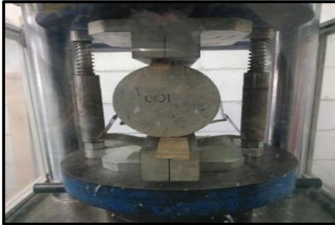
Figure 4. Splitting Tensile strength testing
