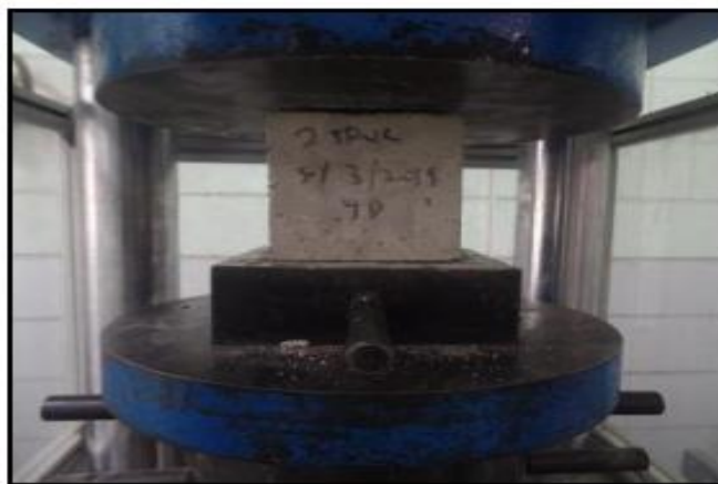
Figure 3. Compressive strength testing
