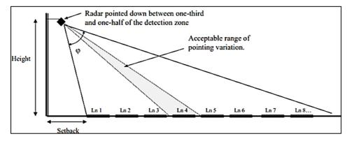
Figure 5. Height of device installation (Houston Radar, 2018).
