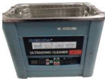
**Figure 6.** Ultrasonic Cleaner for Water Leaching
