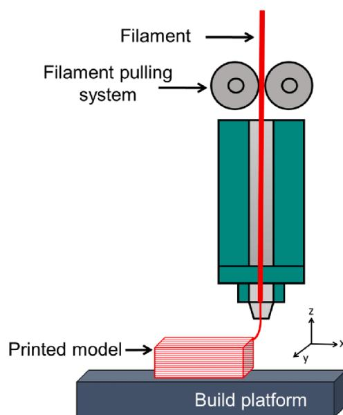
**Figure 1.** Schematic Diagram of FDM
