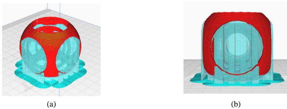
**Figure 4.** Support structure after slicing for mini gyro (a) orthogonal view, and (b) front view.
