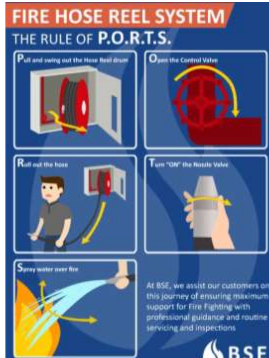
Figure 3.20: P.O.R.T.S rule's to use the hose reel system (BSE, 2019)
