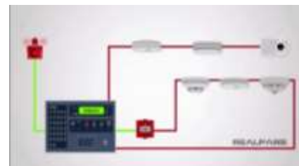
Figure 3.18: the alarm will be making a noise and sends a signal to the control panel
