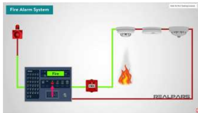
Figure 3.11: the control panel receives a signal from smoke detector and manual call point
