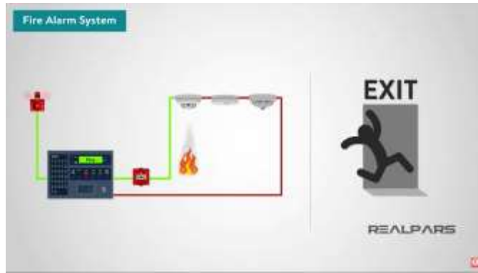
Figure 3.12: the loud noise and the emergency light is activated to warn the personnel and need them to leave the building.
