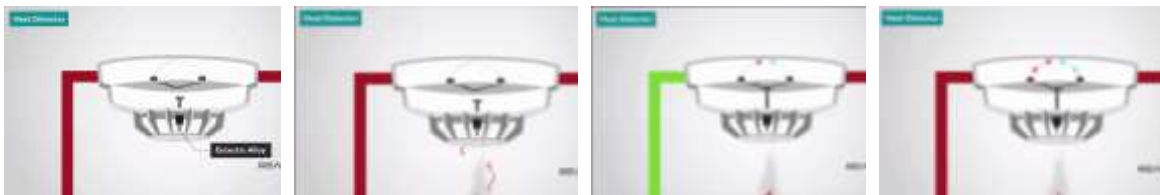
Figure 3.15: The visual of how heat detector works ( https://realpars.com/wp-content/uploads/2019/07/Heat-Detectors-Mechanism.gif#.Ya2WsuxCcRU.link )
