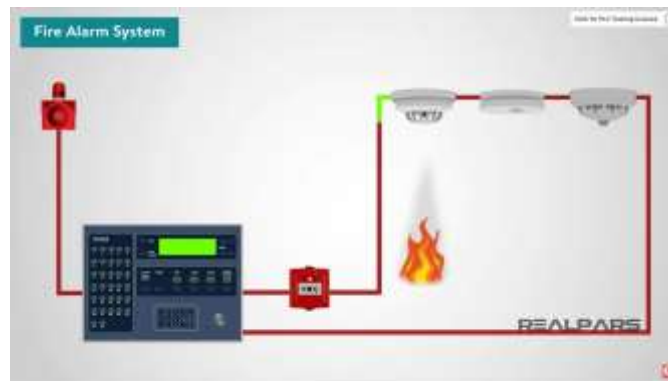
Figure 3.10: the smoke of the flames getting detected by the smoke detector.
