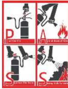
Figure 3.19: The guide to use fire extinguisher.
