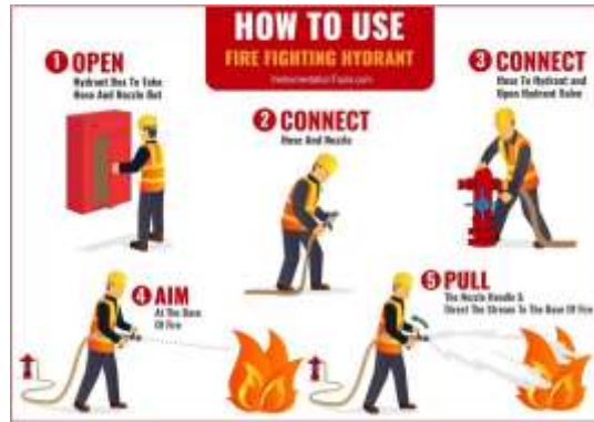
Figure 3.21: a guide to use the hydrant
