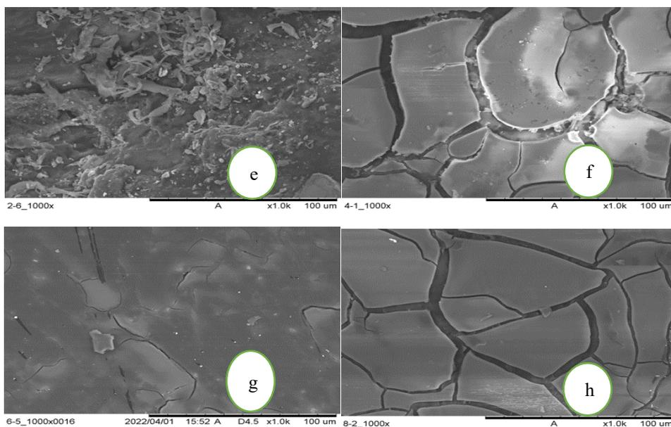
Fig. 2. Polyamide resin surface Photomicrographs using SEM (e-Non coated, f-Brush coated, g-Dip coated, h-Spray coated).
