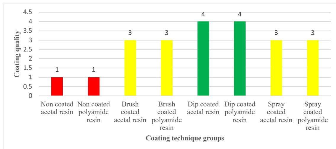
Fig. 3. Surface quality of (non coated, brush coated, dip coated, and spray coated acetal and polyamide groups).
