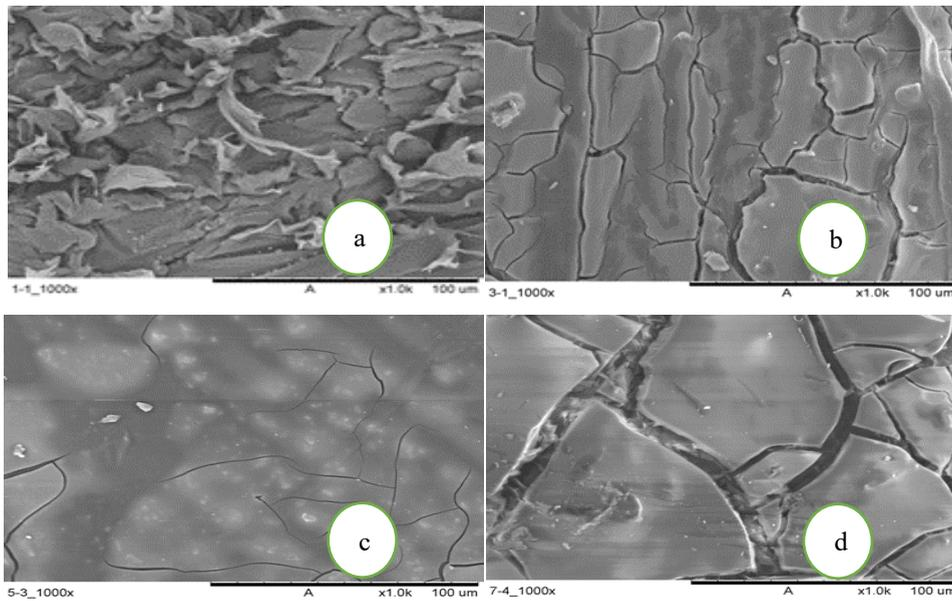
Fig. 1. Acetal resin surface photomicrographs using SEM : (a-Non coated, b-Brush coated, c-Dip coated, d-Spray coated)1000x magnification.
