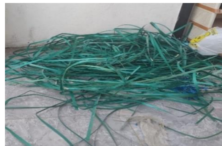
Figure 2. Collecting polypropylene tapes or strips from construction waste.
