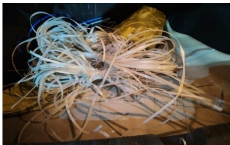
Figure 2. Collecting polypropylene tapes or strips from construction waste.
