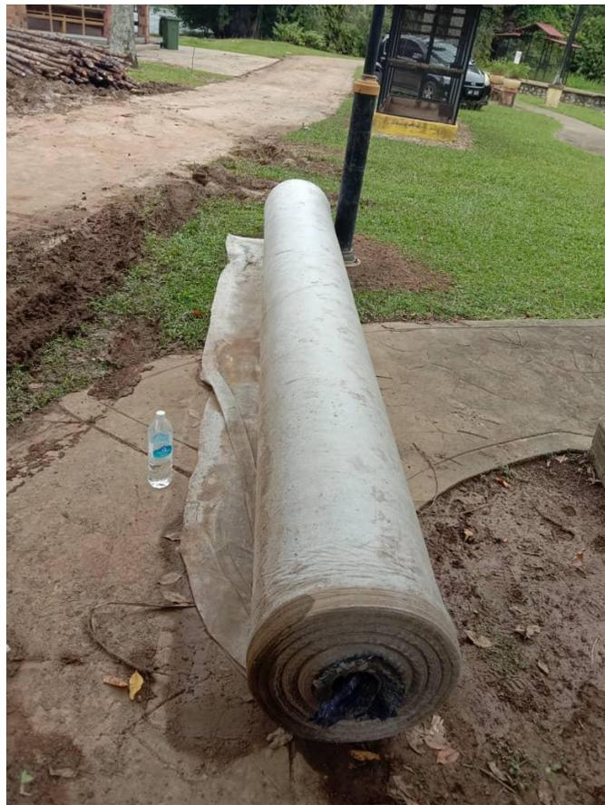
*Figure 3.3.5 Non-woven Geotextile Fabric*
