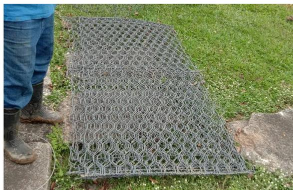
*Figure 3.3.3 Gabion net*
