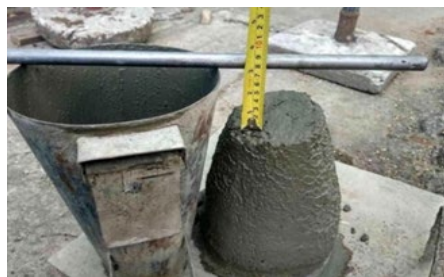
Figure 3.10: Measuring the slump using a measuring tap
