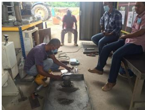
Figure 3.37: Proctor test at the laboratory.
