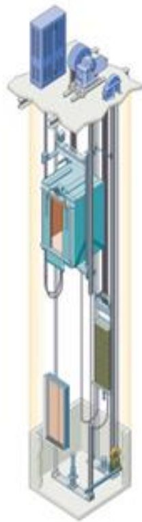
Figure 3.13: Operation of Traction Elevator System
