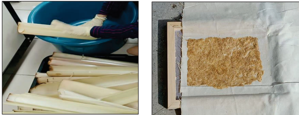
Figure 1. Parts of the manufacturing process of sanitary pads from banana fibres – left: separation of the stem from foliage, right: drying the fibres under the sunlight.
