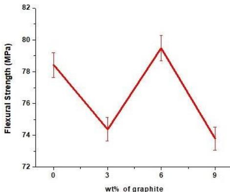
Figure 10: Effect of wt% of graphite in flexural strength of PC/ABS blend
