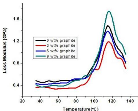
Figure 2: Effect of graphite content in the loss modulus of PC/ABS blend
