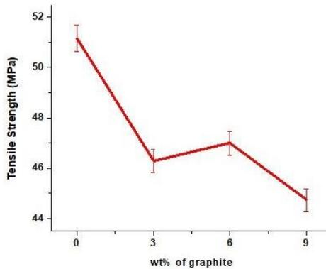
Figure 5: Influence of graphite content on the tensile strength of PC/ABS blend
