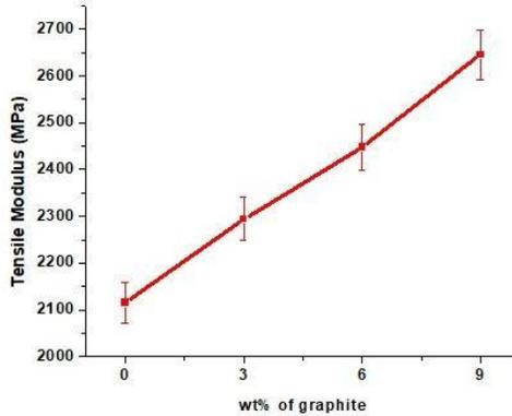
Figure 6: Influence of graphite content in tensile modulus of PC/ABS blend
