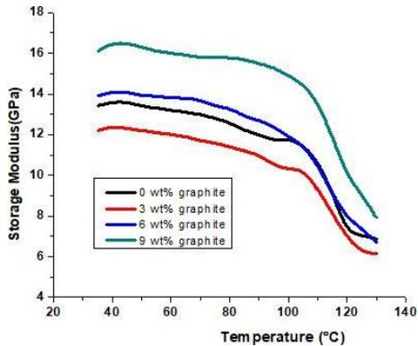
Figure 1: Influence of the graphite filler on the storage modulus of PC/ABS blend
