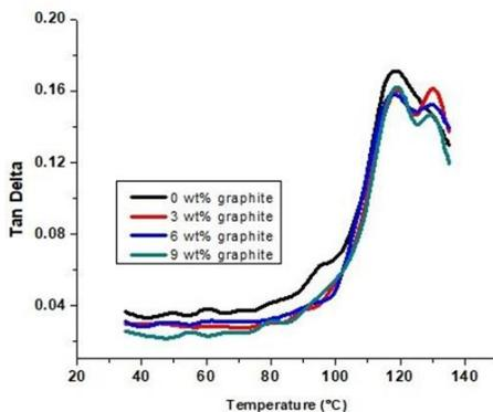
Figure 3: Effect of graphite content in the Tan Delta of PC/ABS blend
