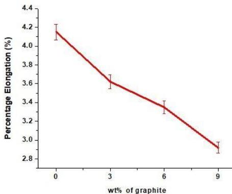
Figure 7: Effect of graphite wt% on the percentage elongation of PC/ABS blend
