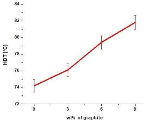
Figure 12: Effect of wt% of graphite on heat deflection temperature of PC/ABS blend
