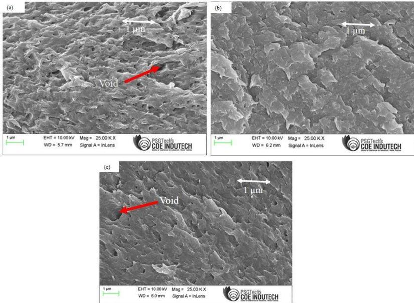
Figure 8: SEM images; (a) PC/ABS and 3 wt% graphite, (b) PC/ABS and 6 wt% graphite, and (c) PC/ABS and 9 wt% graphite
