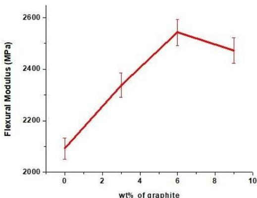
Figure 11: Effect of wt% of graphite in flexural modulus of PC/ABS blend
