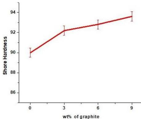
Figure 9: Effect of wt% of graphite in shore hardness of PC/ABS blend
