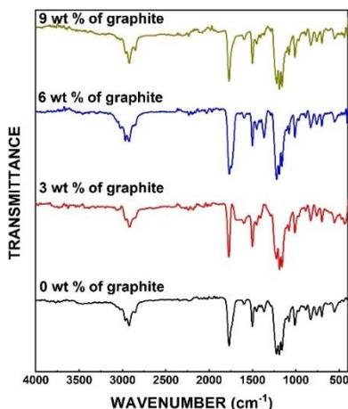
Figure 4: FTIR spectra of neat PC/ABS and the PC/ABS/graphite composites
