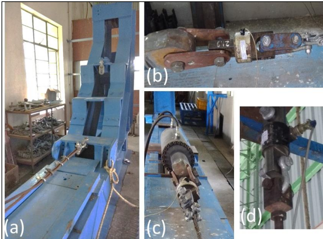
Figure 4: (a) Conductor fixed end sling arrangement, (b) loading end hydraulic cylinder connected with a load sensor, (c) double ended hydraulic cylinder with load-cell and sling, and (d) transverse load sensor and turn buckle arrangement
