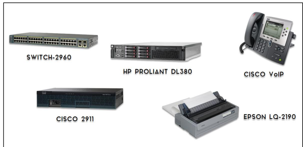
Figure 2.3 List of Network Equipment
