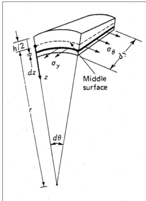
Figure 1.1: Thin Shells' Surface Cross Section.
