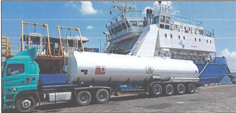
Figure 16: Bunkering operation by ATTSB road tanker for Sapura vessel
