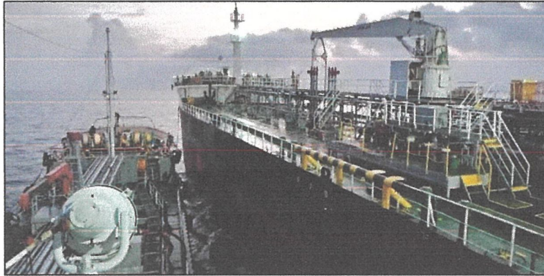
Figure 17: Ship-to-Ship (STS) services alongside on each vessel
