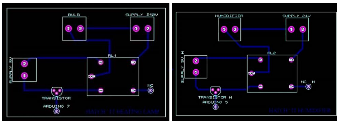
(a) (b) Figure 4. The PCB layout (a) Heating lamp (b) Humidifier
