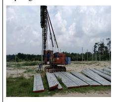
A machine that been use to penetrate the pile into the ground.
