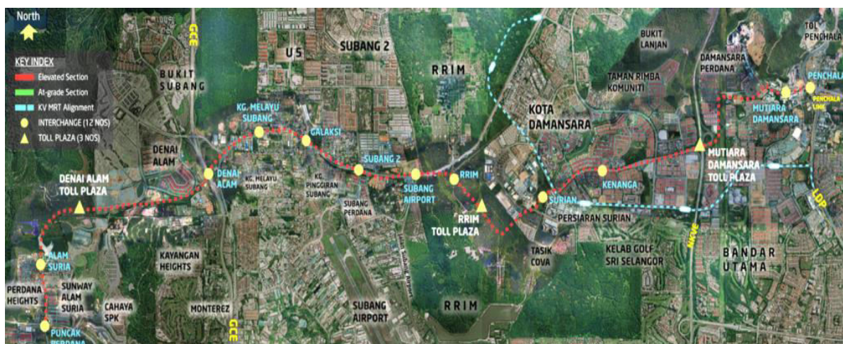
Figure 9 : Full alignment of Damansara-Shah Alam Elevated Expressway
