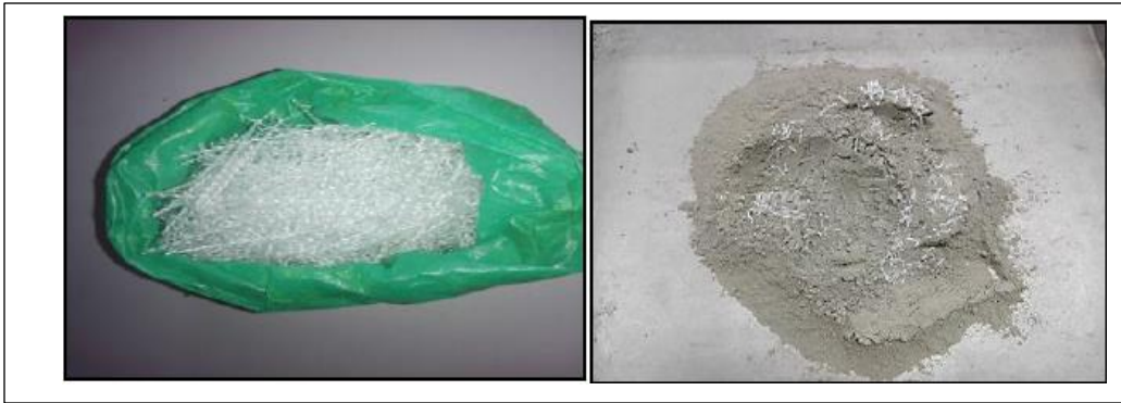
Figure 1. Plastic fiber used as soil-reinforcement (left), Plastic fiber mixed with soil sample.
