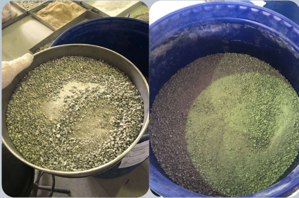
The RCA that passed through the 5 mm sieve was stored in containers
