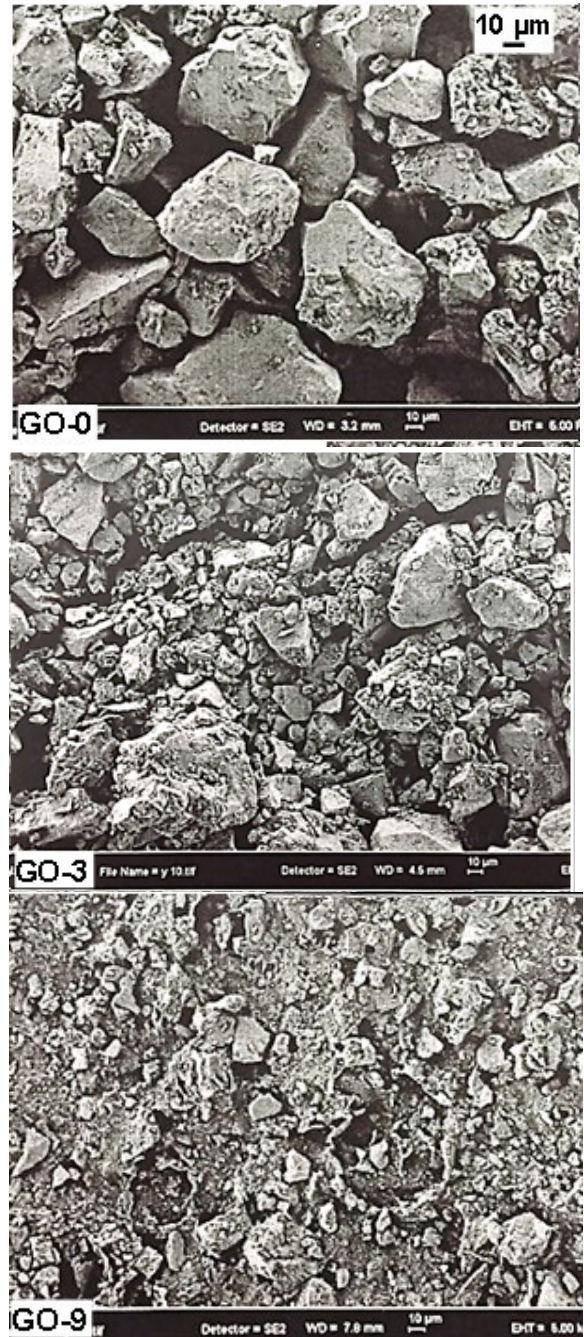
Fig. 9: SEM images of WBDF filter cakes without GO (GO-0), with 3 mg (GO-3), and 9 mg of GO (GO-9)
