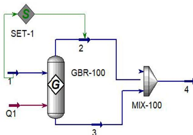
**Fig. 2:** Process flow diagram using ASPEN Hysys
