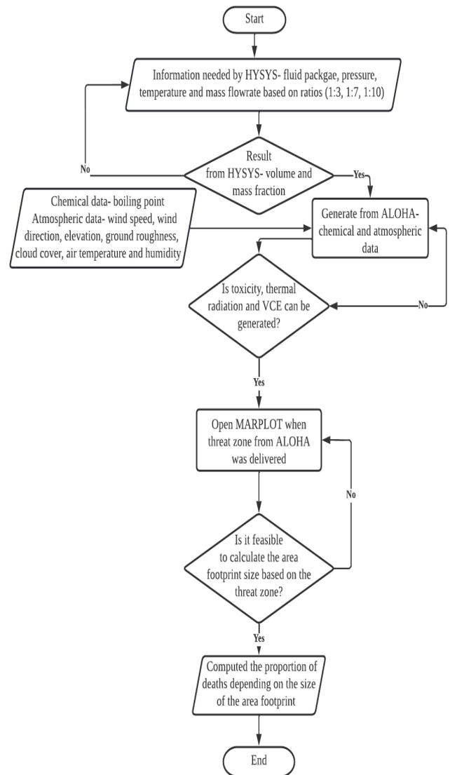
Fig. 6: The flowchart for the process output
