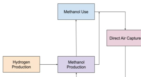
Fig. 1: Flow for CCU route
