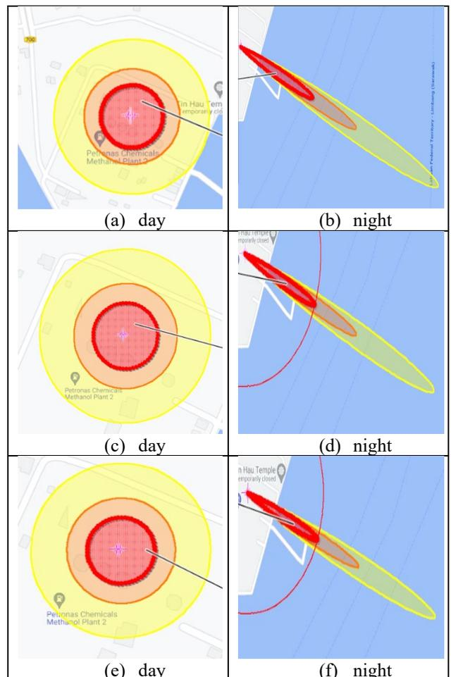
**Fig. 7:** The trace of methanol dispersed in the ratios of 1:3,1:7, and 1:10 throughout the day and night out from the WNW direction of the wind; (a) 1:3, day, jet fire, (b) 1:3, night, toxic, (c) 1:7, day, jet fire, (d) 1:7, night, toxic, (e) 1:10, day, jet fire, (f) 1:10, night, toxic
