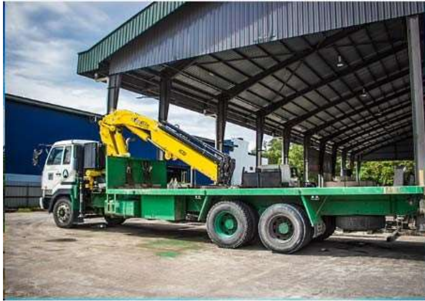
Figure 15: 8-ton lorry crane to transport pile machine and RC Pile
