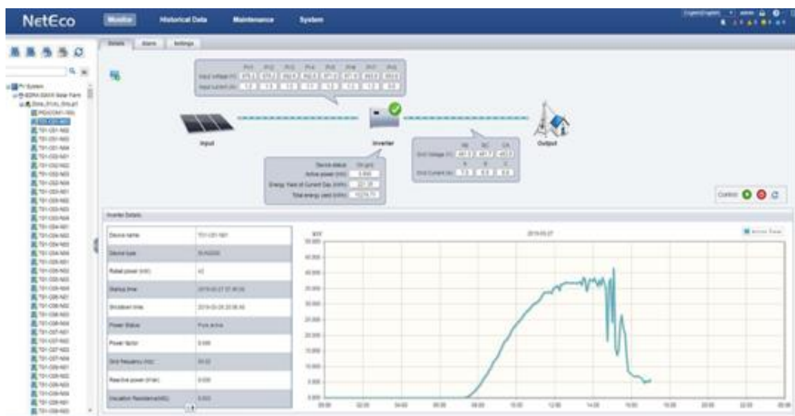
Figure 7: String inverter HMI facilities
