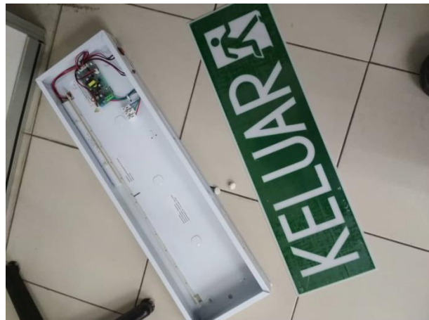
Figure 12: Emergency exit sign 'Keluar'
