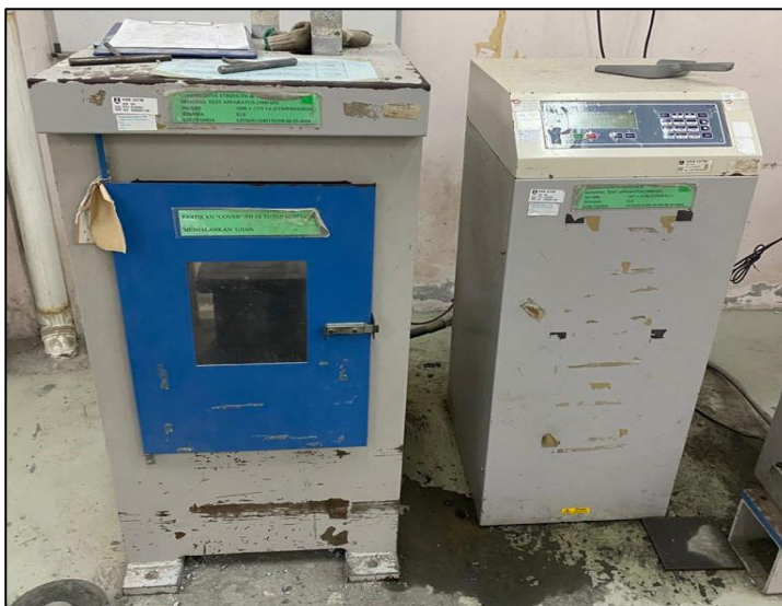
Figure 2. Compressive Strength Machine at UiTM Concrete Lab
