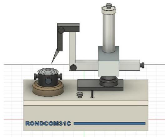
**Figure 2.** Model of roundness measuring machine
