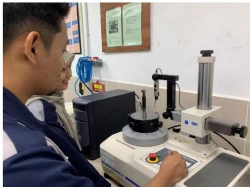
**Figure 3.** Conducting roundness measuring machine using AR system
