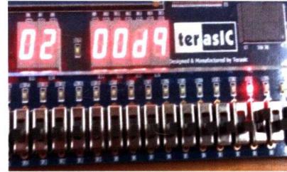
Fig.10 Example output of SDRAM display on FPGA
