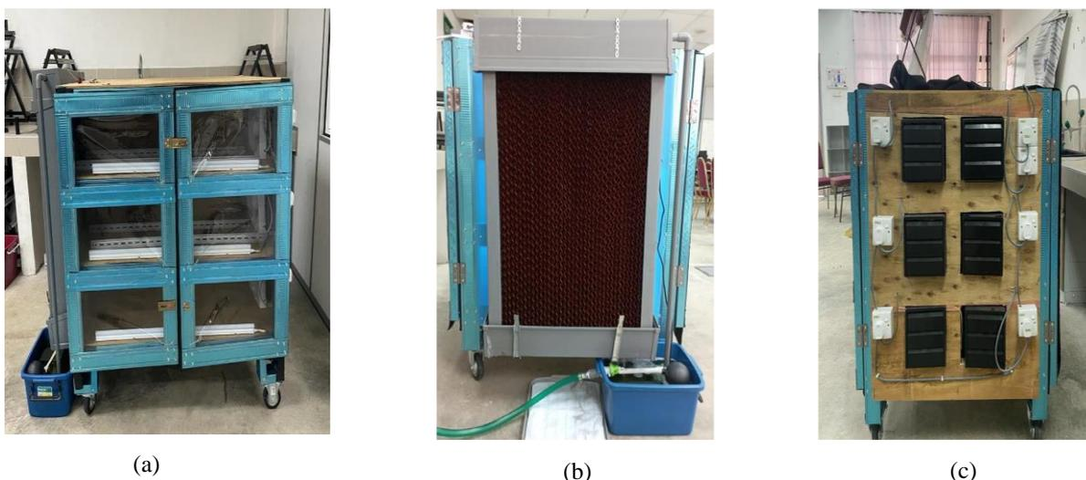
Figure 1: Images of the mushroom chamber with evaporative cooling pad system: (a) front; (b) left; (c) right
