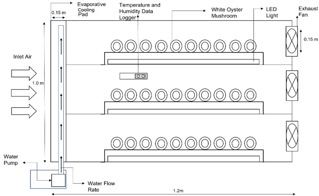
Figure 3: Schematic diagram of mushroom chamber
